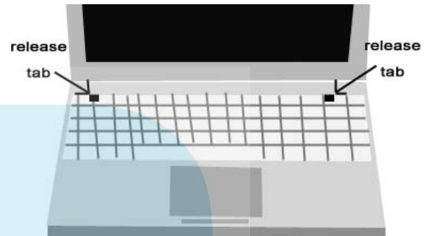
Figure 5-1: The keyboard release tabs.
